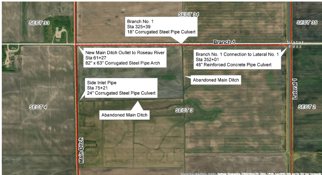
Figure 4. Abandoned Main Ditch Alignment and Associated Structures – Plan View
