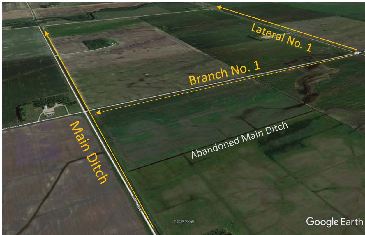
Figure 3. Google Earth Aerial of the Abandoned Main Ditch crossing Section 3, Ross Township – Isometric View
